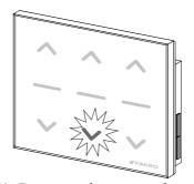
**5\***. Programming error – button flashing for 2-3 sec. as presented in the drawing.
