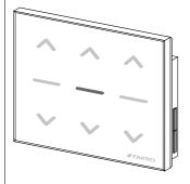
4. The controller is signalizing that the device has been successfully associated (button light up for 2-3 sec. as presented in the drawing).
