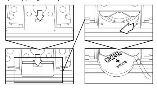
3. Put the battery into position paying attention to the correct polarisation. Position the tape for removing the battery in a way enabling sliding the battery out again with the use of this tape.
