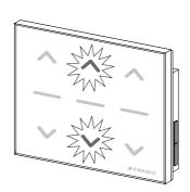
**5\***. Programming error – buttons flashing for 2-3 sec. as presented in the drawing.
