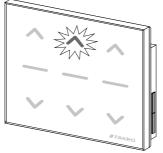
**5\***. Programming error – buttons flashing for 2-3 sec. as presented in the drawing.
