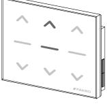
4. After few seconds, the controller is signalizing that associating with the network has been successfully completed (buttons light up for 2-3 sec. as presented in the drawing).
