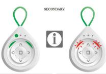
Procedure performed correctly. D1 LED and GREEN backlight is on for a while and then goes off. Error. D1 LED goes off, RED backlight flashes 3 times. Repeat procedure or see page 14, point 1 or 5.
