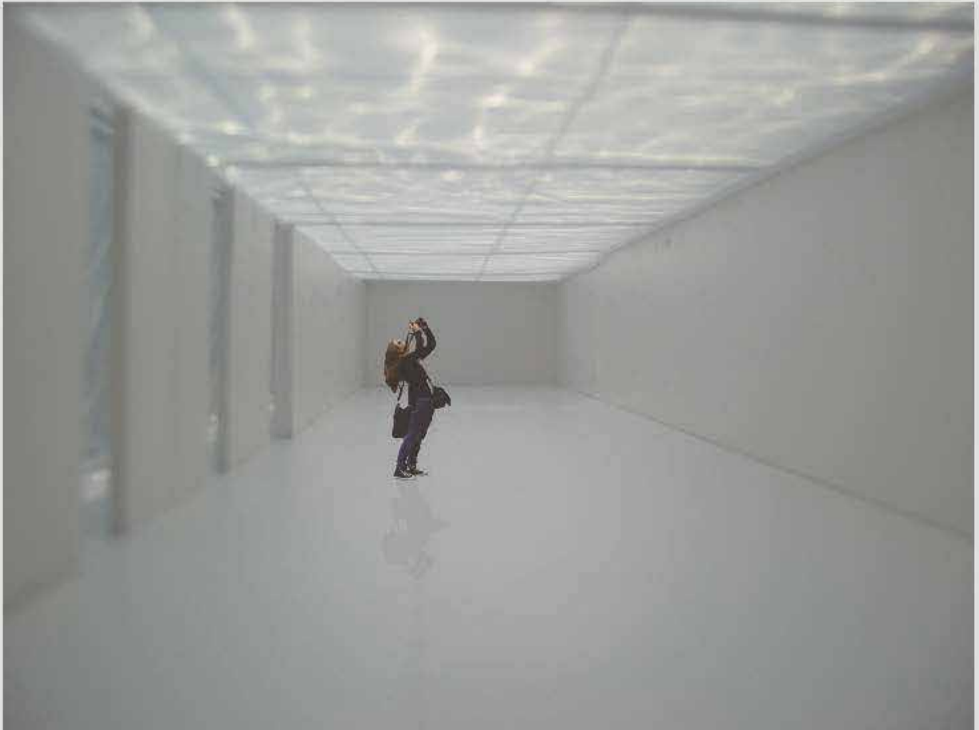
The light through this water membrane illuminates the space without any flickering. Yet, the surface of the membrane, which is the ceiling, has a flickering image caused by the various flows of water.
